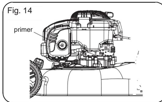
2. Stand behind the mower. Pull the Engine On/Off Control Bar toward upper handle with one hand and place the other hand on the Engine Start Handle.
