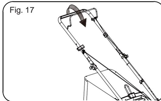
Release the Engine On/Off Control Bar. It will return to its initial position and the engine will automatically switch off.
