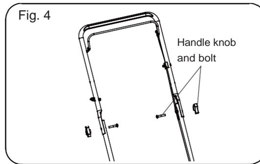
**IMPORTANT:** Unfold handle carefully to avoid pinching or damaging the bowden cable.
