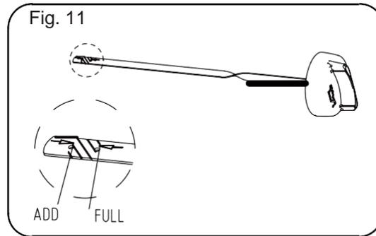
4. Attach oil filler dipstick and tighten by hand.
