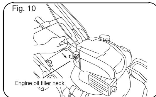
2. Insert the dipstick into the oil filler neck, and tighten it.
