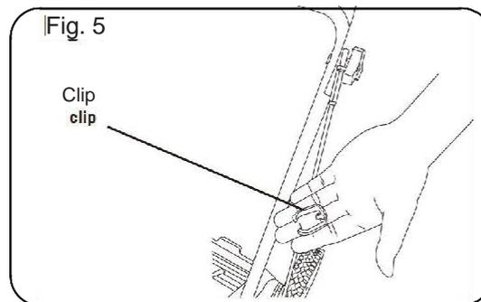
Attach the bowden cable to the lower handle with the cord clip (supplied).
